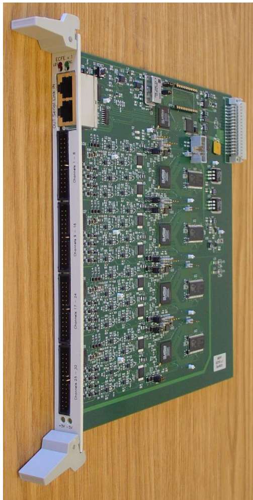
Figure 10: Wire chamber module
