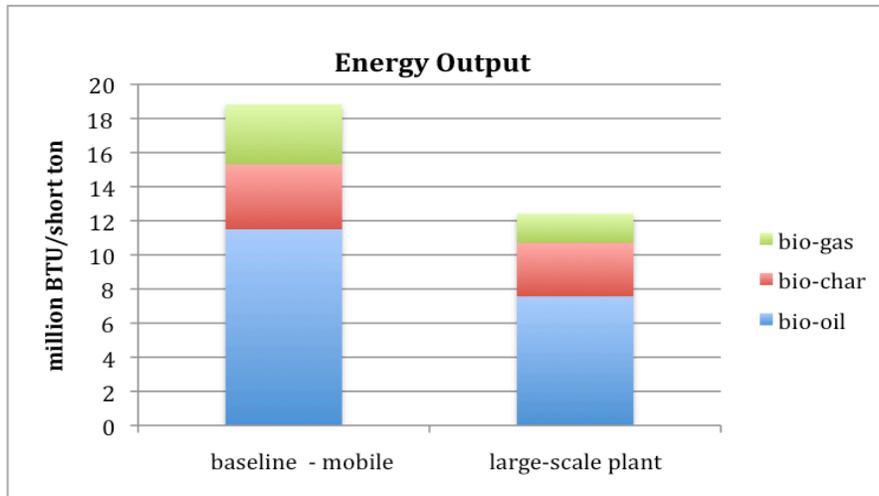
Figure 5. Output energy based on mobile unit and plant unit. The mobile unit estimation is based on Agri-Therm’s woody biomass energy output. The large-scale plant output is based on PNNL’s techno-economic study [Jones et al., 2009].
