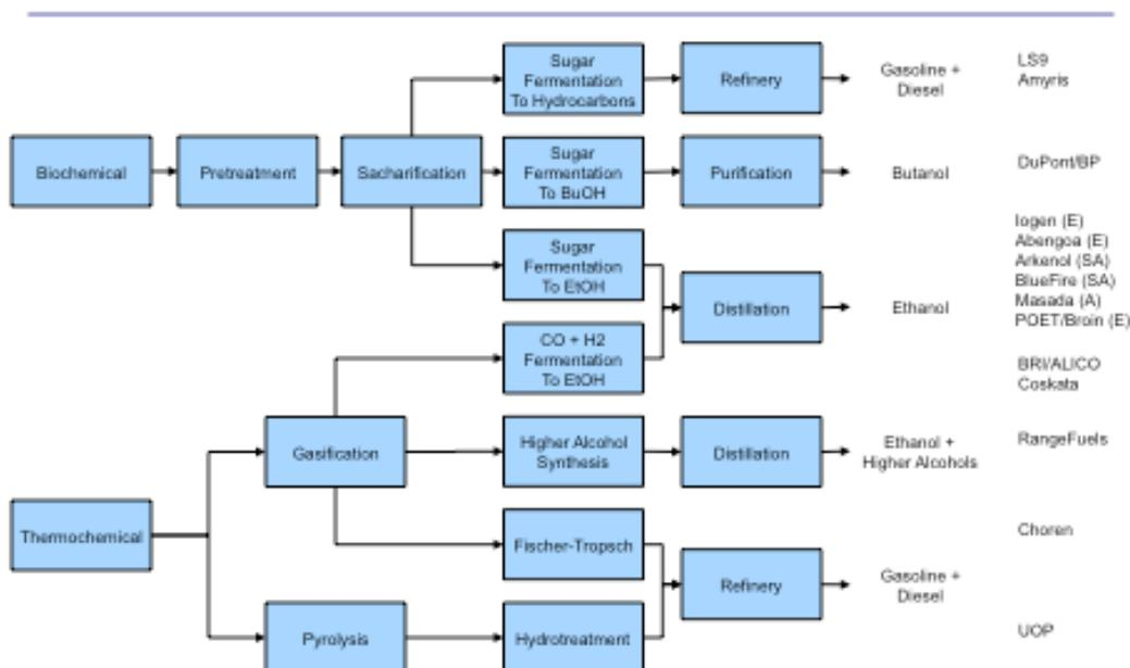
Figure 3. Pathways that lead to different types of liquid transportation fuel. (courtesy of Ben Wu, SNL-CA)
