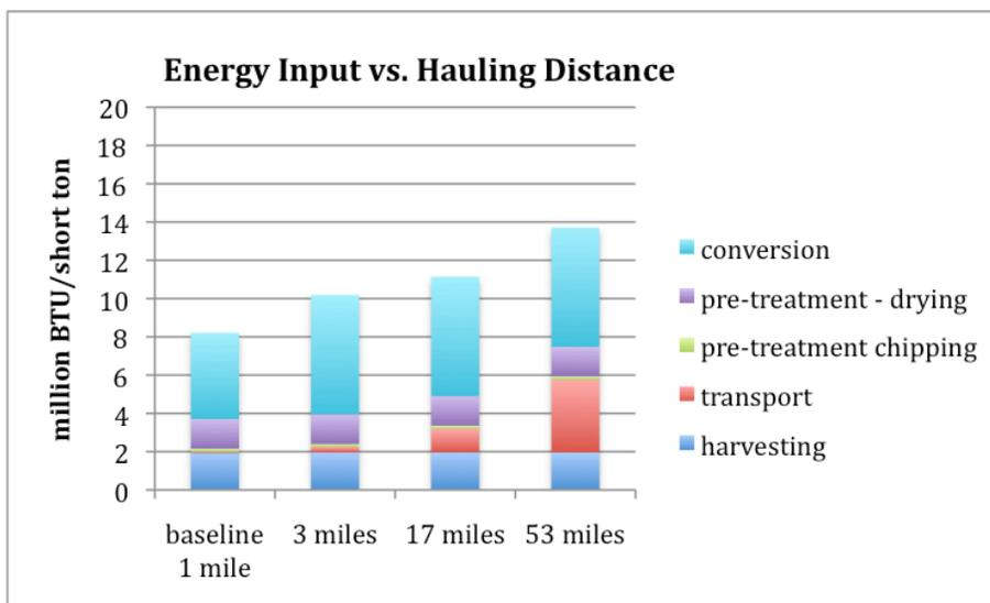
Figure 6. Sensitivity of total energy input as a function of hauling distance
