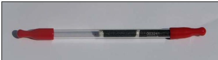
Figure 6-6. Sorbent Trap Used for Trace Metals Testing.
