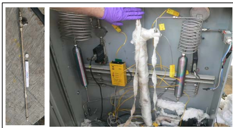
Figure 6-5. MPT Carbon Molecular Sieve Membrane Installed at PSDF.
