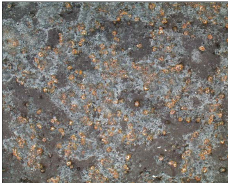
Figure 5-8. Iron Aluminide Filter Media with 10,938 Gasification Hours.
