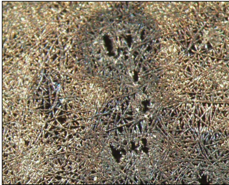
Figure 5-10. Coarse Fiber HR-160 Dynalloy Filter Media with 2,698 Gasification Hours.
