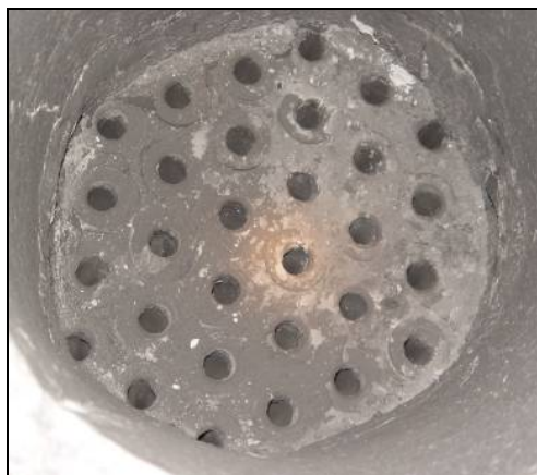
Figure 3-20. Inspection of Primary Syngas Cooler Inlet Tubesheet.
