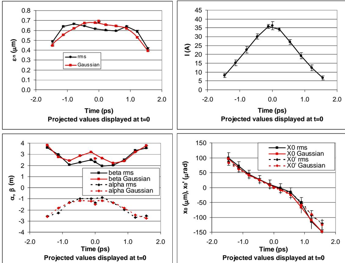
Figure 10: The emittance versus time is plotted in the upper left and the  $\alpha$  and  $\beta$  functions at the initial point are shown in the lower left. The current versus time is shown in the upper right based on the total charge and the charge contained in each slice. The measured offset angle and position at the initial point are shown in the lower right corner. The measurement of the projected beam is plotted at  $t = 0$  on all graphs.
