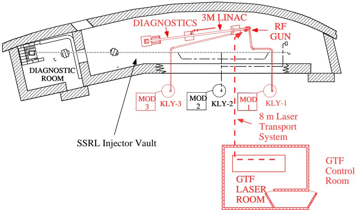
Figure 1: The Gun Test Facility at SLAC.
