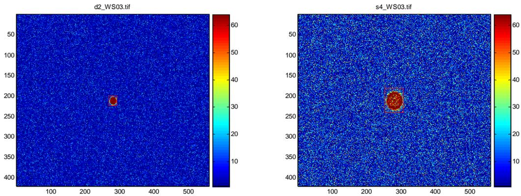
Figure 12: Two images at screen location three generated from the simulation code PARMELA. The image on the left has 20  $\mu\text{m}$  pixel size and 60 counts of average noise level with standard deviation of 10. The image on the right has 10  $\mu\text{m}$  pixel size and 100 counts of average noise level with a standard deviation of 20. The red boxes are the ROI for each image as calculated using the algorithm described earlier.
