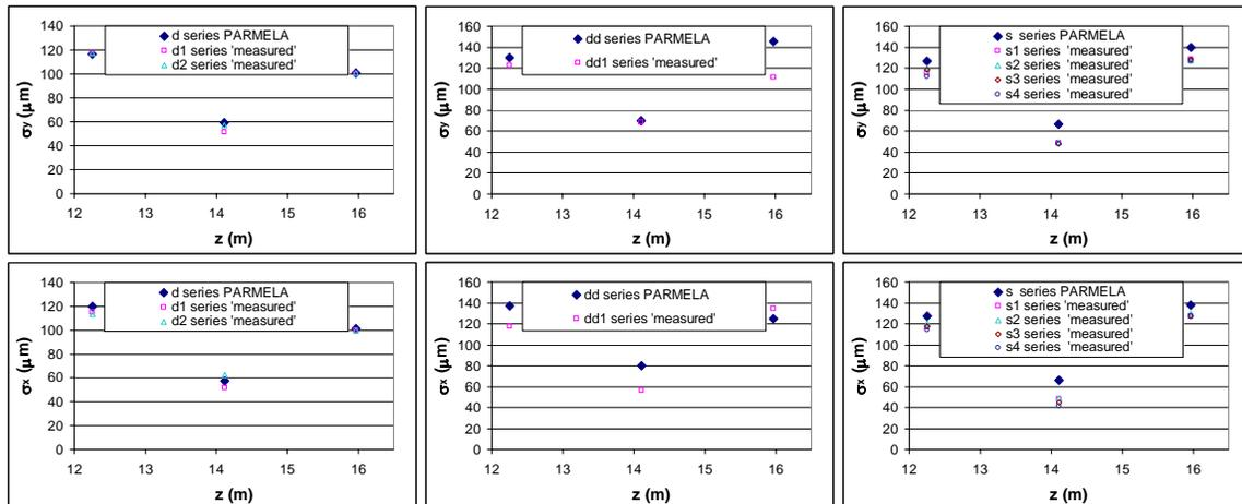
Figure 13: The horizontal rms beam size is shown on the bottom row and the vertical rms beam size on the top row for three different sets of beam parameters. Several different test cases for each set of beam parameters were run with different pixel size, average and standard deviation noise level.
