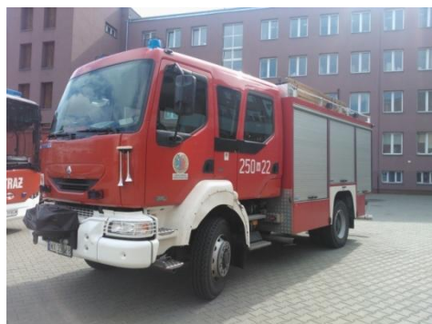
Fig. 1. Medium rescue – firefighting vehicle with chassis manufactured by: a) the Renault Midlum, b) the Mercedes-Benz
