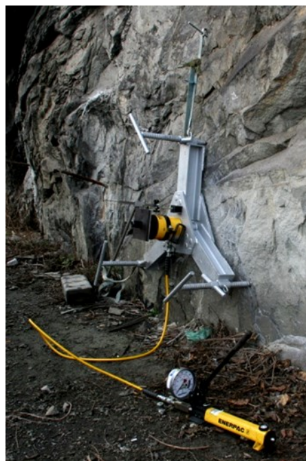
Fig. 1 Loading stand with hydraulic system
