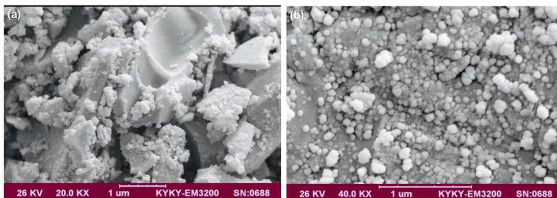
Figure 1. SEM image of (a) Fe 3 O 4 -NPs-AC and (b) Au-Fe 3 O 4 -NPs-AC
