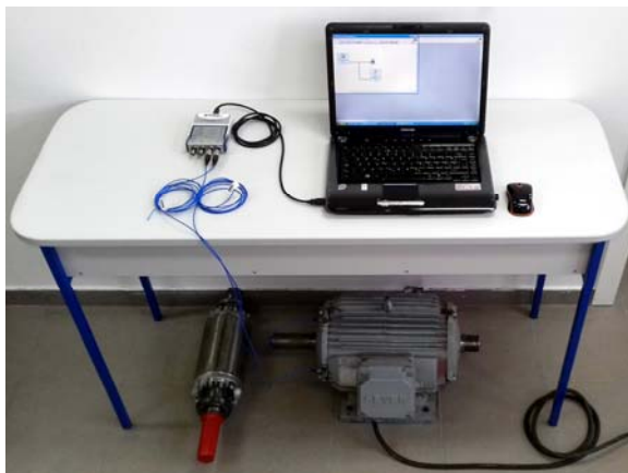
Figure 2. Laboratory setup for broken bar detection based on vibration signals
