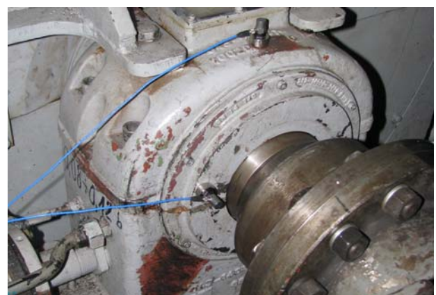
Figure 5. Shear accelerometers with magnetic mounting
