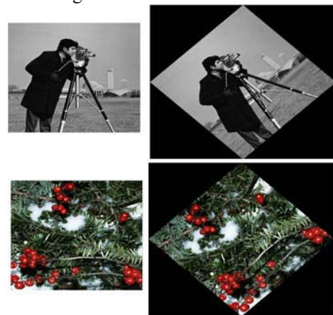
Figure 6. Image rotation using precalculated tables: rotation angle is 45^\circ
