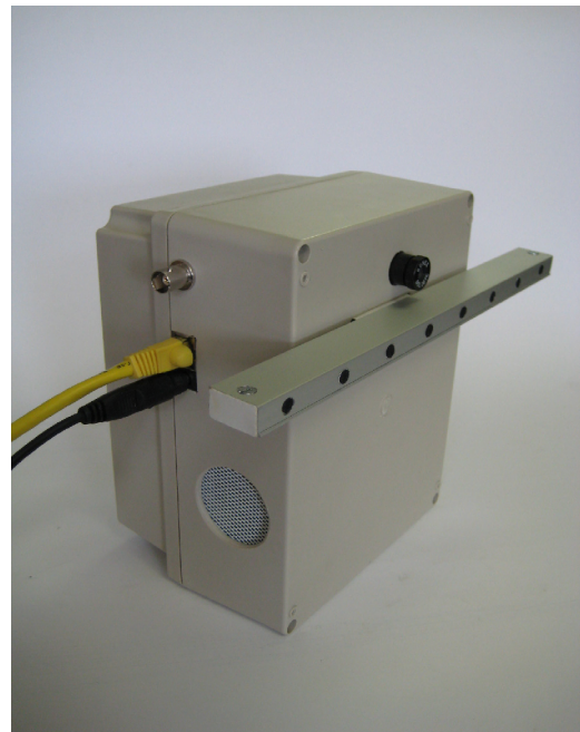
Figure 6. The node, with apparent camera and microphone array.
