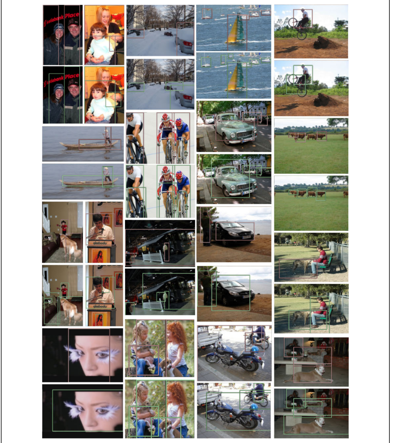
Figure 13. Detection results of some testing images on VOC 2007 26 data set. The results of BING 14 are shown in odd rows (pink boxes), and the corresponding ones of proposed method are displayed in its next row (green boxes).
