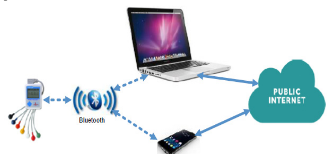
Figure 3. Transmitting data through the Bluetooth interface
