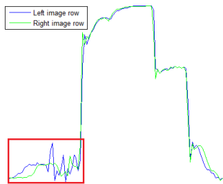
Figure 3. Red rectangle highlights the discontinuity between two superimposed profiles
