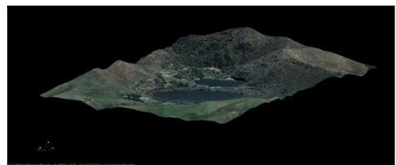
Figure 4. Example of points clouds performed by aerophotogrammetric method with 1 meter resolution
