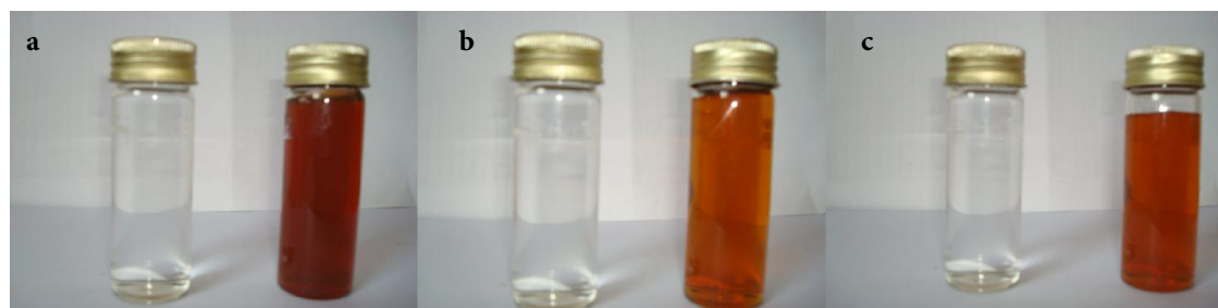
Figure 1. Color change during synthesis of silver nanoparticles. Silver nitrate (colorless liquid); SNPs synthesized from a) thyme, b) pennyroyal, and c) marshmallow.
