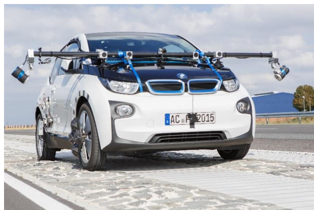
Figure 28: Test drive on Belgian block
