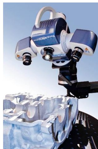
Figure 20: Scanning of a crankcase
