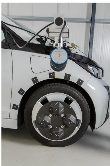
Figure 27: Test preparation: Camera, wheel adaptor and reference on fender
