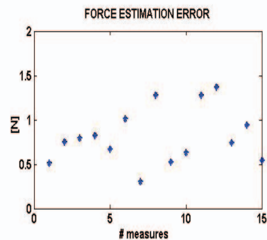
Figure 8. Mean error between the force measured by the force/torque sensor and the force computed by the electric current.
