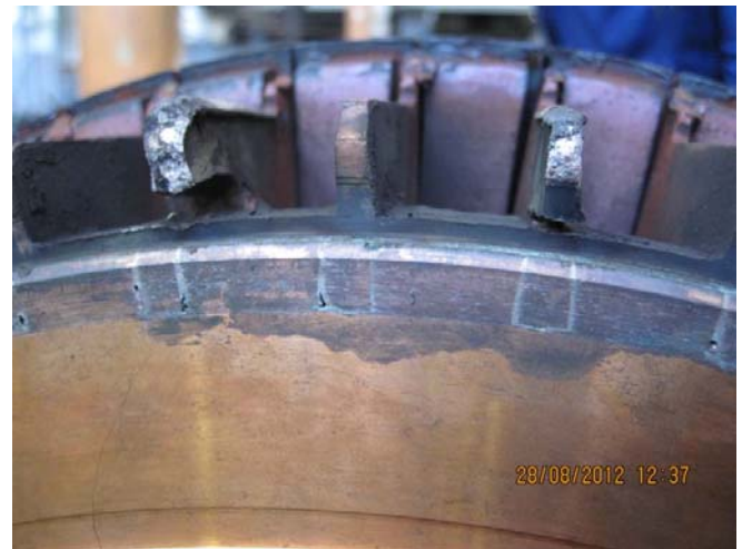
Figure 11. Visual inspection of dismantled rotor confirmed the existence of two cracked rotor bars
