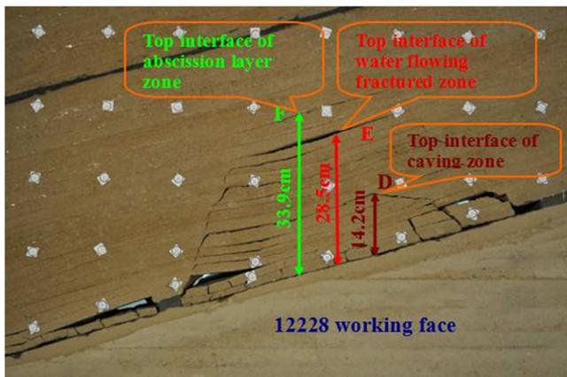
Fig. 6. Failure status of overlying rock mass after excavating the 12228 working face.
