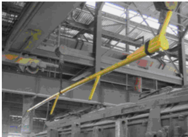
Figure 12. Albras non metallic air fluidized conveyor of three outlets
