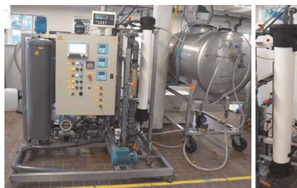
Figure 1 | The pilot-scale FO set-up and the SWFO membrane module at the KWR pilot facility in Nieuwegein.
