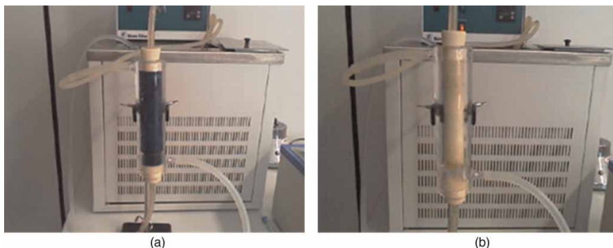
Figure 5 | Anoxic reactor packed with PUF cylinder. (a) Before and (b) after the decolorization.
