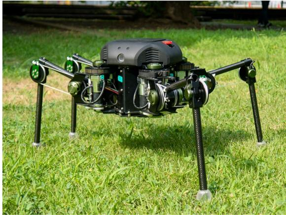
**Fig. 2** Sprawling-type quadruped robot TITAN-XIII
