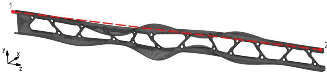
Figure 3. First local buckling mode.
