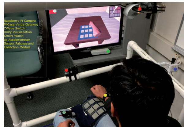
Figure 1. The figure shows our prototype system and experimental setup demonstrated by a subject. The system is composed of a four by three capacitive sensor array sewn into the denim fabric using conductive wires. The data from the sensors are analyzed using our custom-designed wireless module, which uses capacitance measurement ICs, an MSP430 micro-controller, and Bluetooth wireless module. It also demonstrates the Smartwatch accelerometer, which was used to profile gestures for confidence and intensity. The visualization demonstrates two kinds of feedback; instantaneous positional data, and post-gesture classification.
