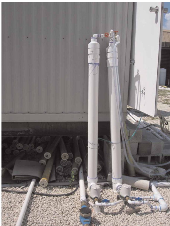
Figure 3 | Lime and kiln dust filters.
