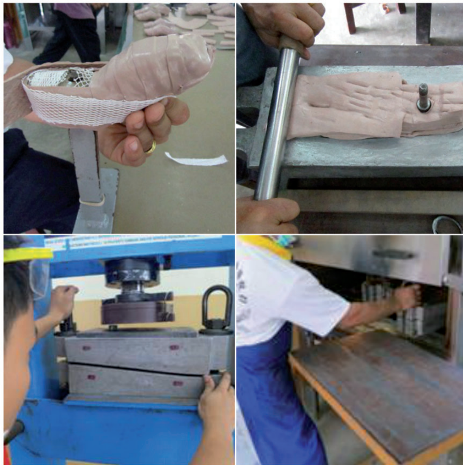
Figure 4. Foot manufacturing process and vulcanization.
