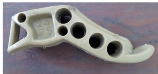
Figure 1. Keel of the prosthetic foot.
