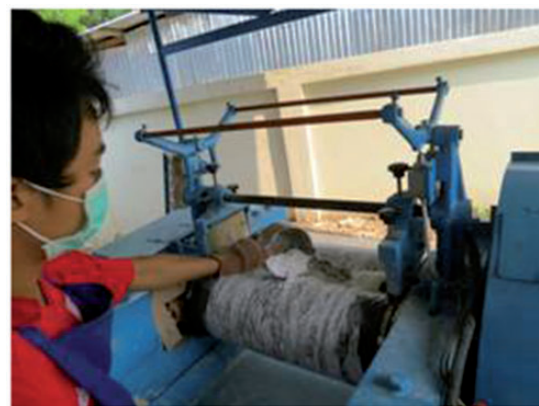
Figure 2. Rubber mastication process.
