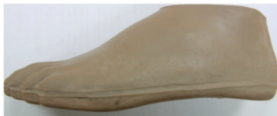
Figure 5. The modified natural rubber CR SACH foot.
