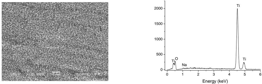
**Figure 2:** Micrographs and EDS spectrum of a Na-Ti layer.
