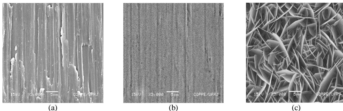
**Figure 1:** Micrographs of surfaces: (a) cp Ti, (b) Na-Ti and (c) Ti-OCP.
