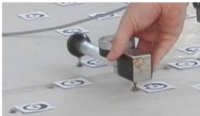
Fig. 4 Location of coded RAD targets and metal markers for determining the strain in the radial and tangential directions.
