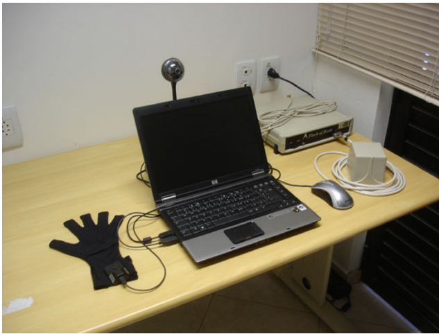
Fig. 1 Hardware setup—data glove, laptop/webcam and motion tracker (not used for the current experiments)
