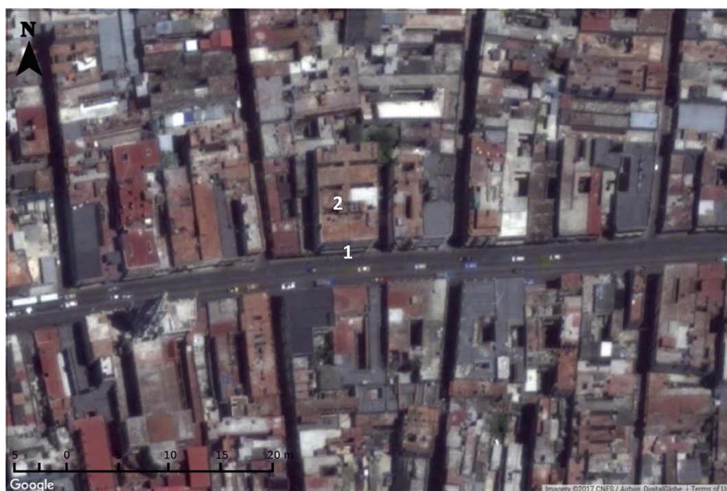
Fig. 1. Data collection site (Simon Bolivar Street). 1: Thermo-Scientific ADR 1500 profiler and traffic video recording. 2: AIRDAM anemometer. Adapted from Google Earth.
