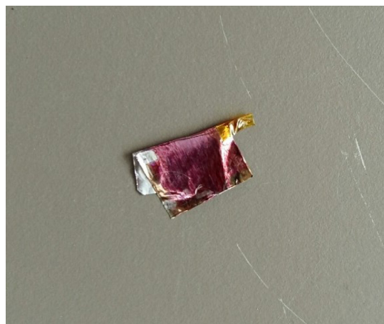
Fig. 3. Photo of FeFET fabricated on Al foil substrate and folded.
