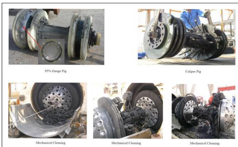
Figure 6: pipeline inspection and mechanical cleaning
