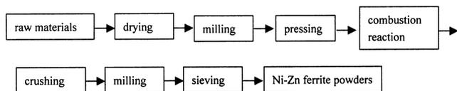
**Figure 2.** The flow chart of SHS process.
