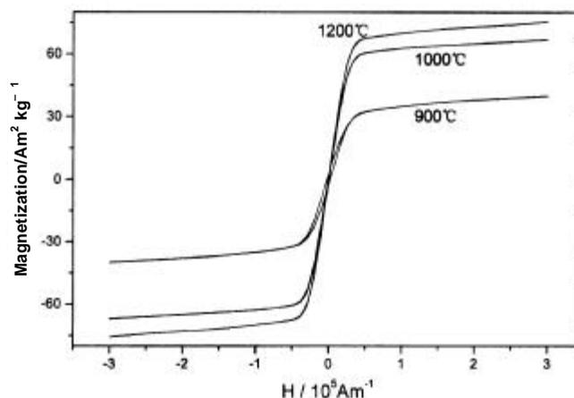
Figure 9. Hysteresis loops for SHS ferrite powders prepared at different combustion temperatures.
