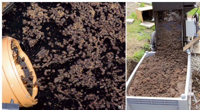
Fig. 4. (a) Floating faeces with cork granules (lighter, reddish particles) entering the outlet pipe and (b) faeces being collected and transported by the surface separator to a sludge box
