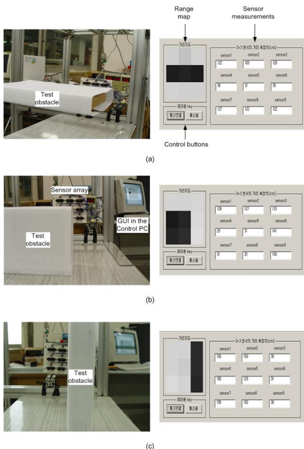
Figure 8. Obstacle detection. (a) Horizontal bar at 30 cm distance and IR sensor measurements, (b) Case of a rectangular object, (c) Case of a vertical object
