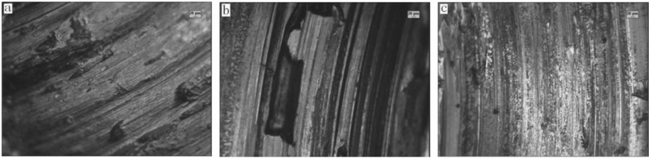
**Figure 7.** Micrographs of steel balls for (a) original abrasive surface and abrasive surface repaired by (b) base oil or (c) nanometer  $WS_2$ .
