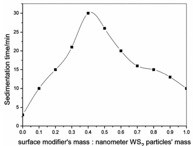
Figure 4. Variation of sedimentation time of particles in base oil with content of surface modifier.
