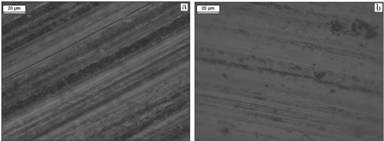
**Figure 9.** Micrographs of piston ring for (a) original abrasive surface and (b) abrasive surface repaired by nanometer  $WS_2$ .
