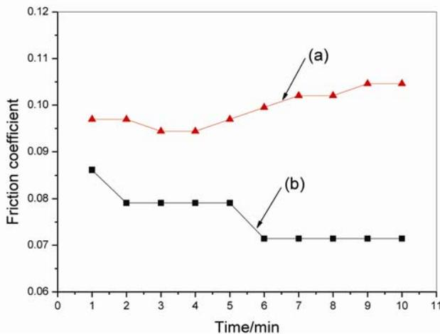
**Figure 8.** Variation of friction coefficients of (a) base oil and (b) the oil including nanometer  $WS_2$  with time (load: 392N).
