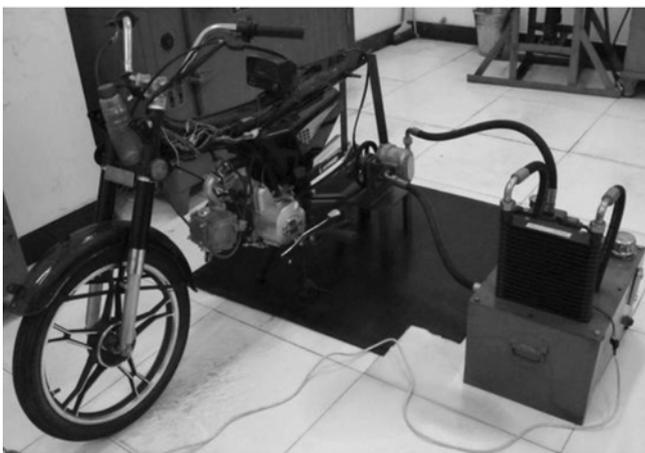
Figure 3. Photograph of engine lubrication test-bed.
