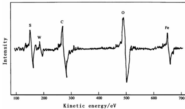
**Figure 10.** Auger electron energy spectrum of abrasive surface repaired by nanometer  $WS_2$ .
