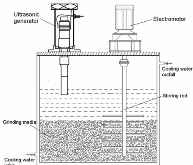
Figure 2. Schematic diagram of dispersing equipment.
