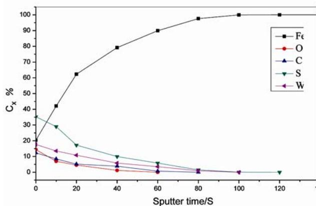
**Figure 11.** Depth distributing curves of elements on abrasive surface repaired by nanometer  $WS_2$ .
