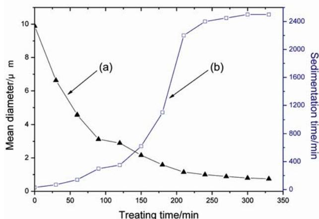
Figure 5. Variation of (a) mean diameter and (b) sedimentation time of particles in base oil with treating time.
