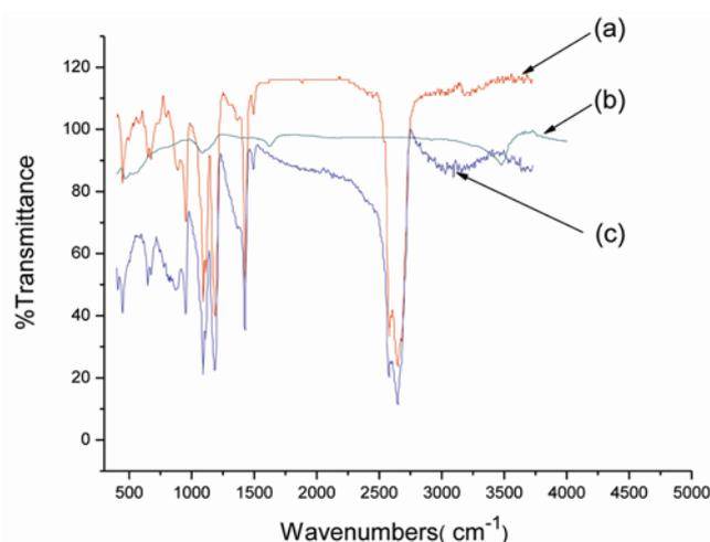
Figure 6. Infrared spectrogram of (a) surface modifier and nanometer  $WS_2$  particles and (b) untreated or (c) treated.
