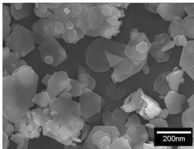
Figure 1. Microcosmic appearance of nanometer WS<sub>2</sub> particles.
