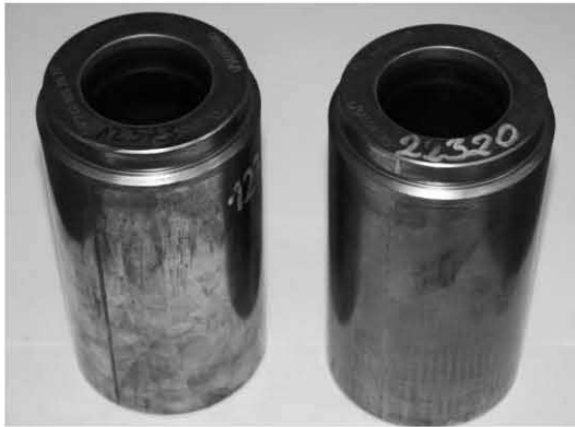
Fig. 10. Optimized tools for forging CVJ casing
