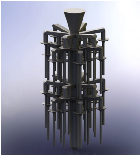
Fig. 5. Investment cast tree with 48 components
