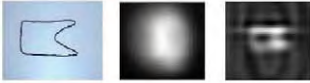
Fig. 22. Close-loop wire (left), the raw metal detector image (centre) and the image after image processing (right).
