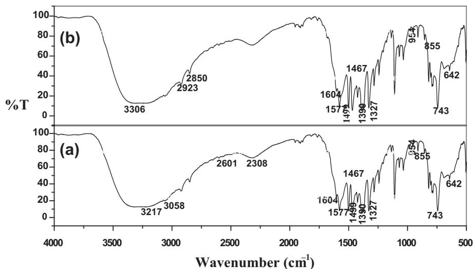
Figure 5. FT-IR spectrum of (a) Znq2 and (b) Znq2:CTAB.
