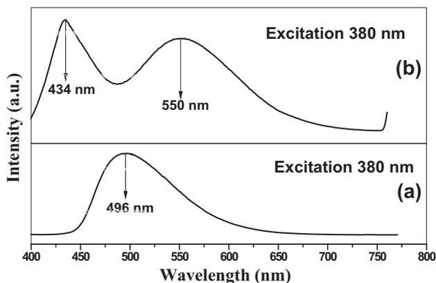
**Figure 7.** Photoluminescence spectra of (a) Znq2 and (b) Znq2:CTAB.
