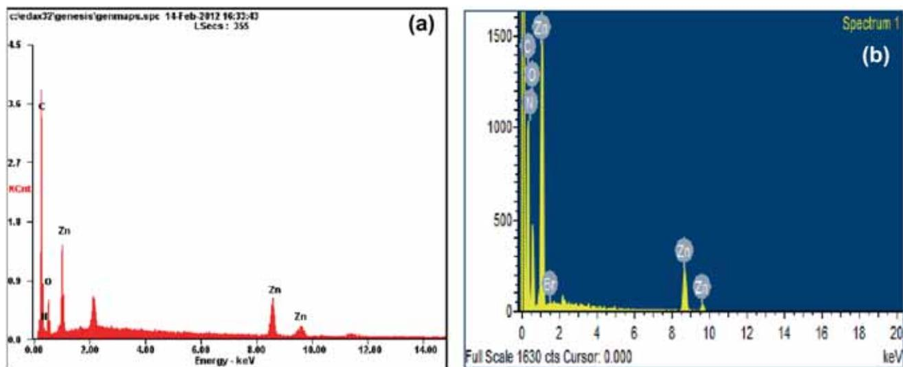
Figure 4. EDAX spectrum of (a) Znq2 and (b) Znq2:CTAB.
