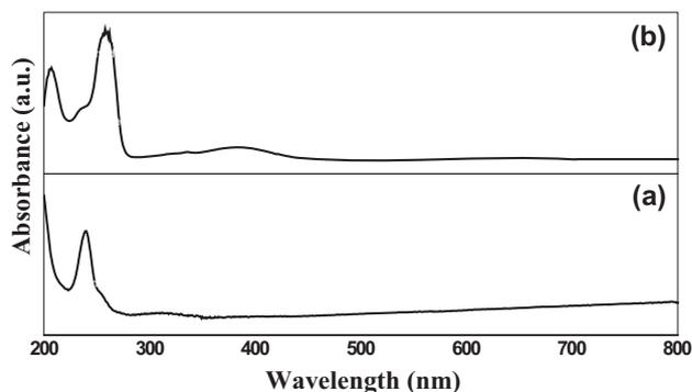
Figure 6. Absorption spectrum of (a) Znq2 and (b) Znq2:CTAB.
