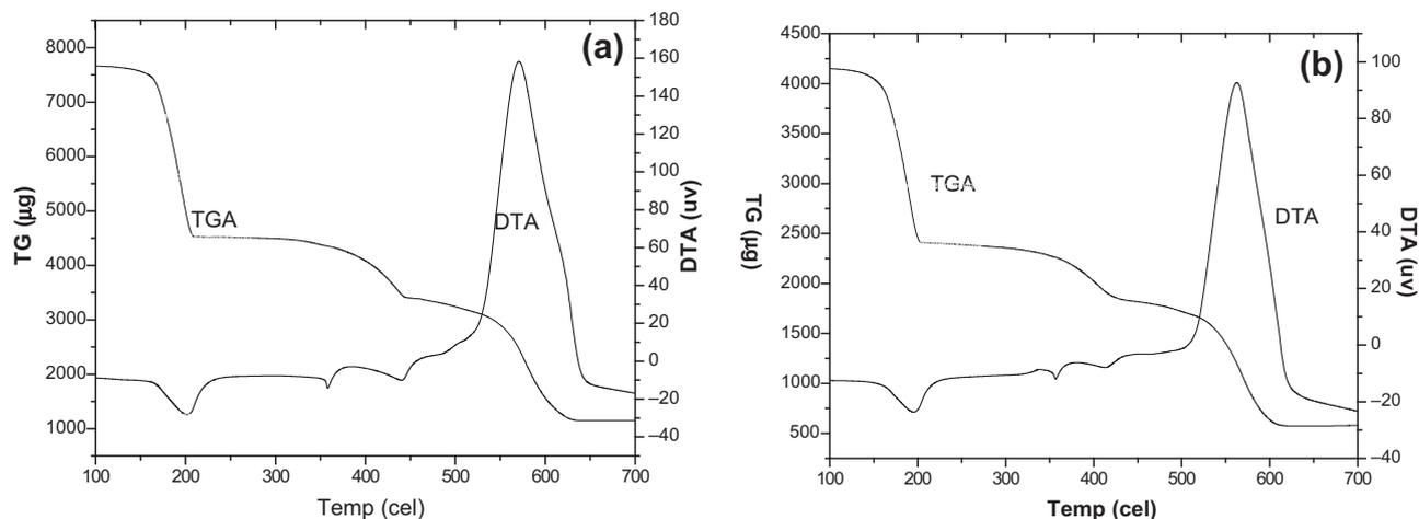
**Figure 2.** Thermal analyses of (a) Znq2 and (b) Znq2:CTAB.
