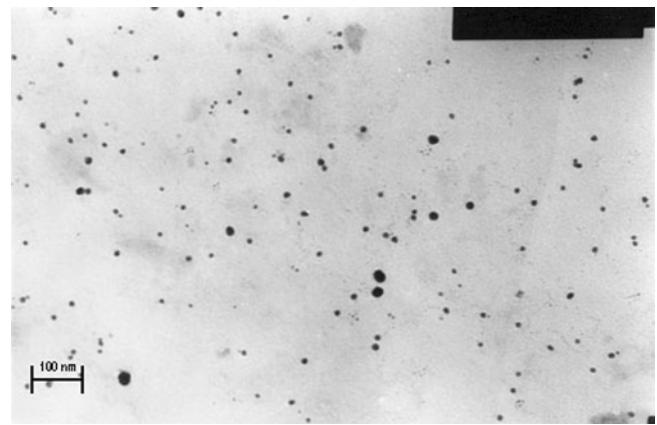
Figure 2. Transmission electron image of silver nanoparticles at 1,00,000  $\times$ .
