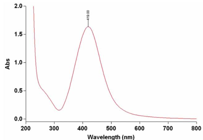
Figure 1. UV-Visible absorption spectroscopy of starch capped silver nanoparticles.
