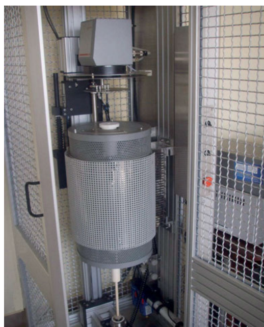
Fig. 3. Photograph of rotational viscometer used in investigations
