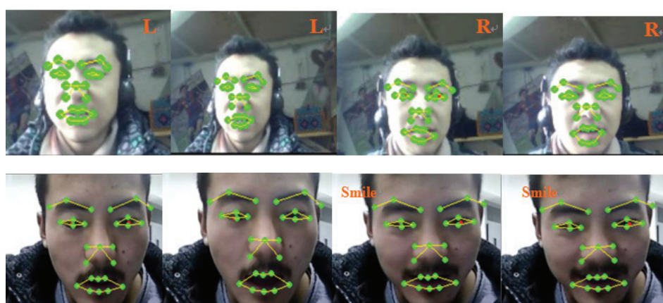
Figure 11. Facial feature point detection and tracking results under different head poses, facial hair, and facial expressions. The tracked points are marked in green and the red letter shows the head pose and facial expression.
