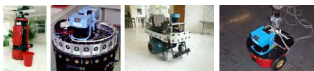
Fig. 1. Different robot platforms operated by SmartSoft reusing many components for navigation skills.
