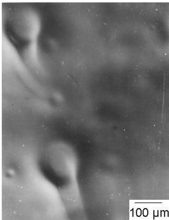
Figure 5. Optical microscopic image of GaAs treated with procedure 2 as described in table 1.
