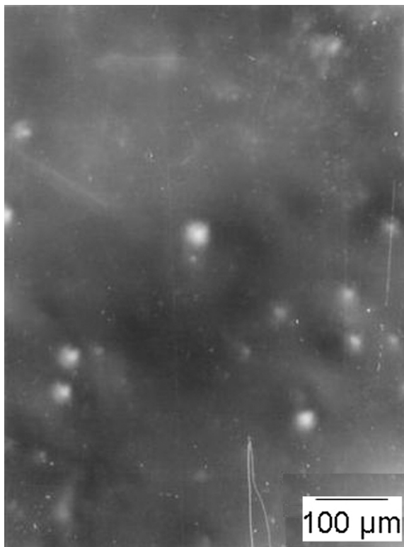
Figure 4. Optical microscopic image of GaAs treated with procedure 1 as described in table 1.
