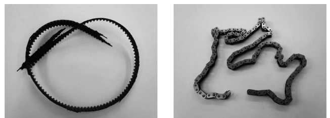
Fig. 4. Damage to belt and chain of timing system
