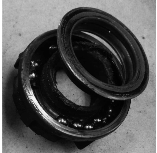
Fig. 7. Worn thrust bearing
