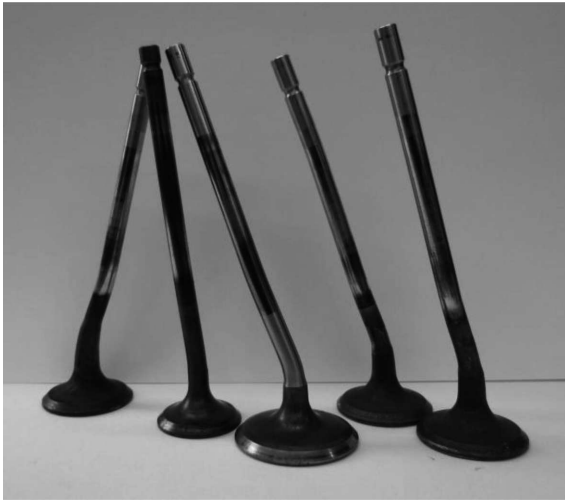
Fig. 5. Distortion of valves
