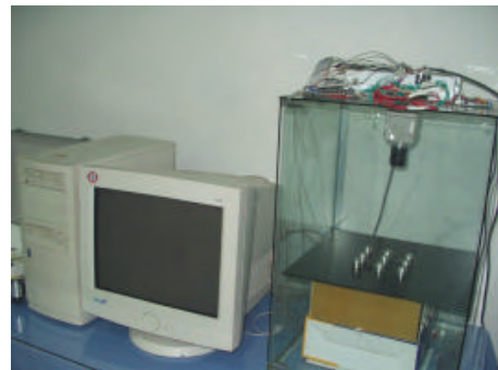
Fig. 10. Microrobot control system based on computer vision
