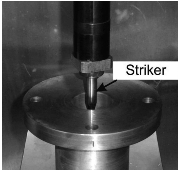
Fig. 1. View of striker and anvil
